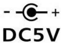
Polarity of DC plug
